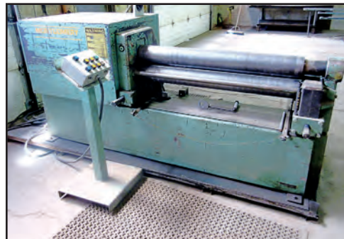
MONTGOMERY 4818-H INITIAL PINCH SHEET ROLLS
